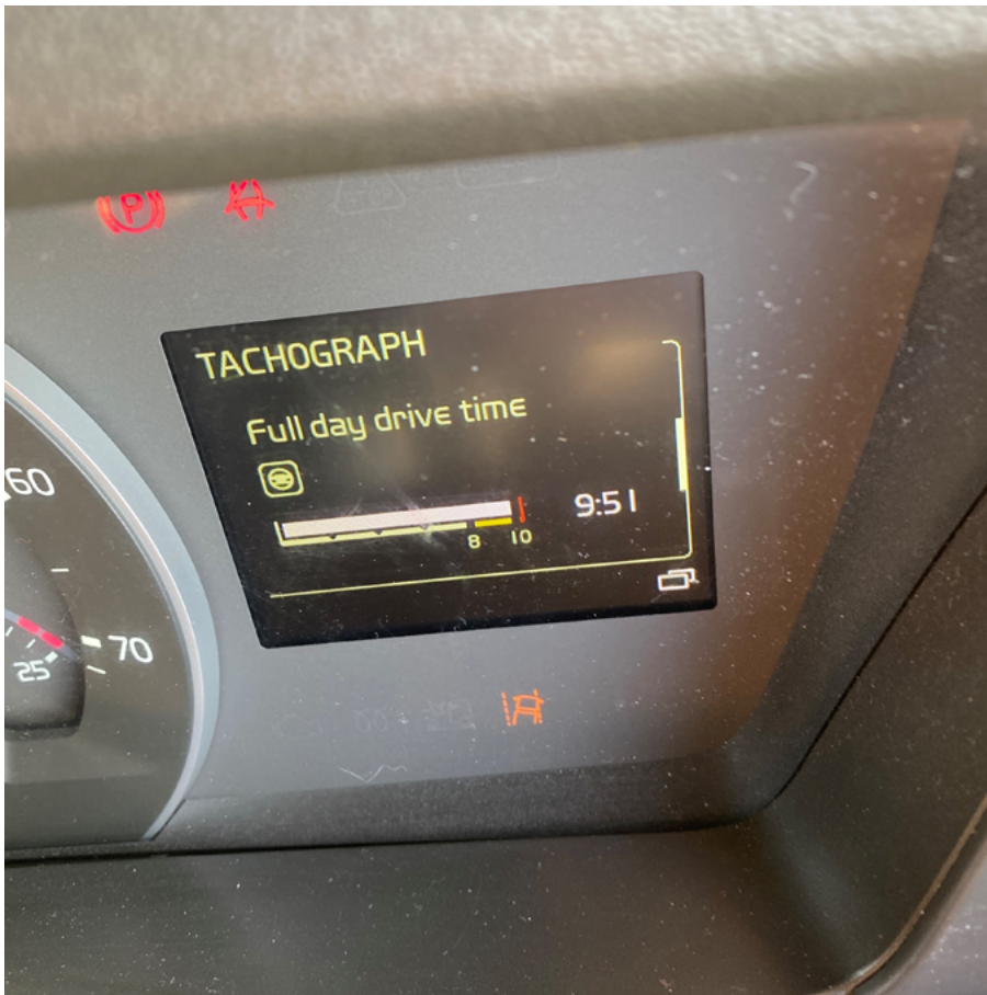
Tacho(graphic) time. Digital tachographs are built into modern trucks, guiding drivers' paid and unpaid time, with financial penalties for infringements.
