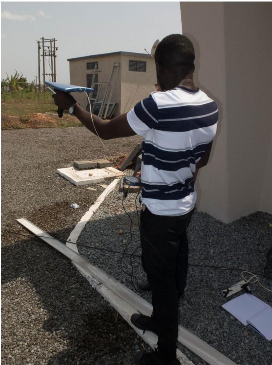
A student in the Development in Africa with Radio Astronomy program detecting radio frequency interference near the Ghana Radio Astronomy Observatory. Photograph: James Merron, June 2018.
